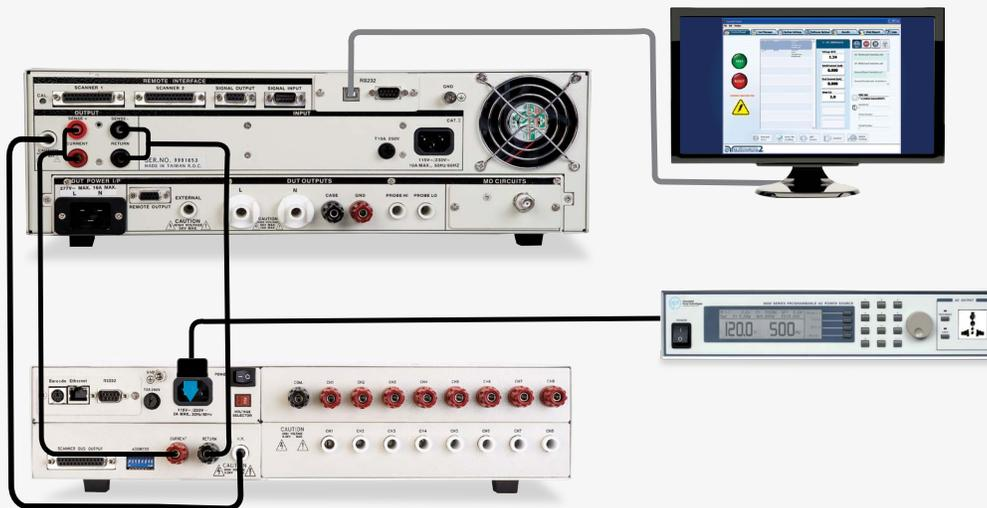
As part of our MedTEST system, we offer high voltage multiplexor. Having your OMNIA II connected to these multiplexors mitigates operator error by automatically switching connection points for each individual test. While the entire test sequence can be set manually through the front panel of the OMNIA II, utilizing software to remotely set and save test sequences is a more efficient method of creating the test sequence.
